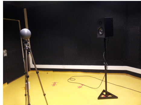
Fig. 3: Experimental setup: plastic sphere and speaker tripods in the acoustic room. Infrared cameras were measuring the ground-true positions.
