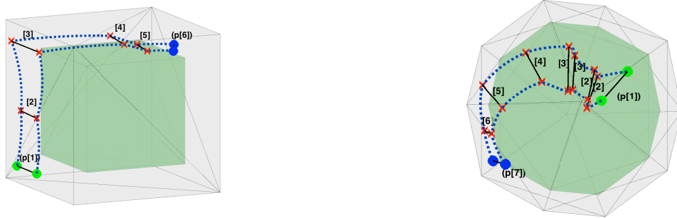
Fig. 4. Example of a smooth trajectory linking the green and blue poses of the 2 fingers end-effector for cubic and spherical bodies. The agent is naturally bypassing the inside of the body where no sensation was generated. Red crosses show known end-effector poses and blue dotted line show interpolated poses along the continuous motor trajectory.
