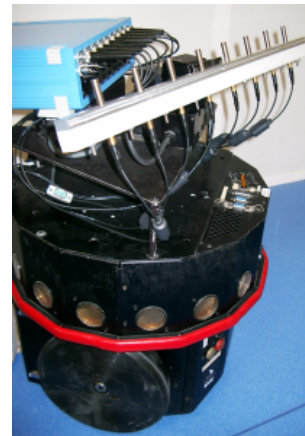
Fig. 1. Experimental Testbed. A 50cm array is being mounted on our SCOUT mobile robot
